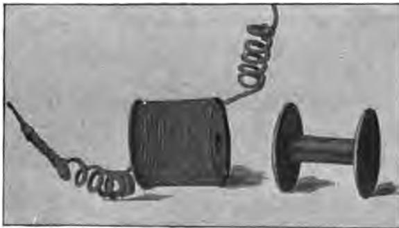
FIG. 39.—COIL OF WIRE WOUND ON INSULATING SPOOL.
